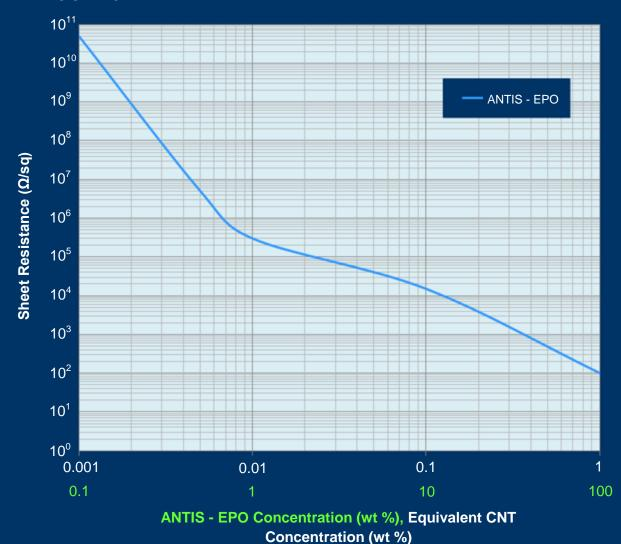
Volume resistivity measurements were conducted using a <100 $\mu$ m (<4 mil) film prepared with ANTIS<sup>TM</sup>-EPO, EPON 828/D.E.R. 331, EPIKURE 3370 curing agent, without pigment. Volume resistivity may vary for different formulations, curing agents, film thicknesses and measurement conditions.
